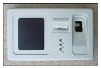
The installation and wiring of a "Combi Proximity Card Reader and Fingerprint ID Reader" into the Access Control system is identical to the "Combi Keypad Reader". The one exception is that each Access Control Power Supply will support only one Combi Proximity Reader, due to power consumption considerations.
