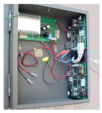
In this picture, the top Access Control Assembly has been wired for one ID Reader and one Relay and has been attached to an Ethernet network. The USB cables from the Fingerprint Reader and the Relay are plugged into the two USB connectors and the Ethernet cable has been plugged into the RJ45 connector of this same Access Controller. All cables and wires are exiting to the right through one of the installed cable glands.
